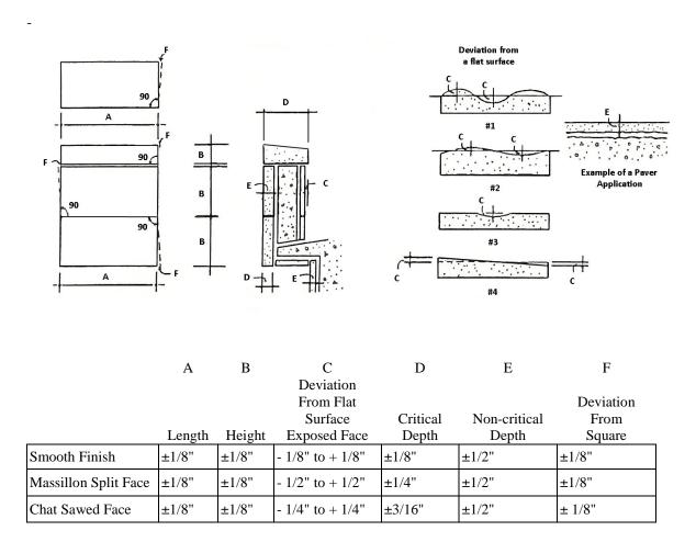
Tolerances C and F are measured within the length of a 4' - 0" straightedge applied at any angle on the face of the stone
